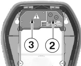
2. Remove the termination panel cover. The termination panel **2** is now accessible.
