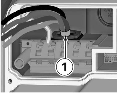
1. Route the supply cable through the cable gland and tighten the gland.
