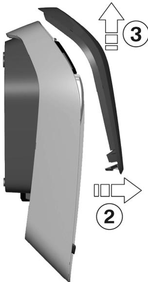
2. Swing the housing cover forwards a little on the underside **2**.
