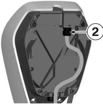
1. Route the supply cable in a loop to the cable gland **2**.
