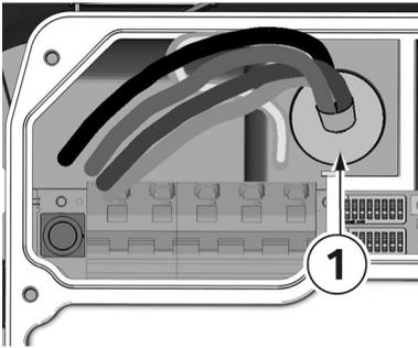
1. The supply cable must be routed through the bushing/double membrane seal **1** as shown in the illustration.
