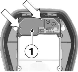
1. Undo the two fastening screws on the terminal cover **1**.
