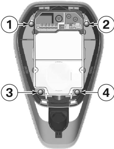
1. After inserting the cable, attach the Wallbox to the two top wafer-head screws **1** and **2**.
