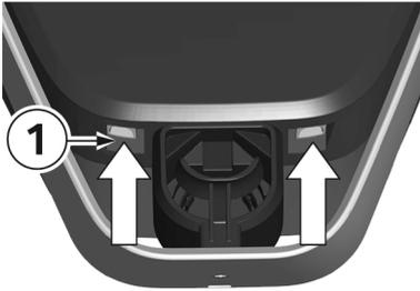
1. Press the two interlocks **1** for the housing cover on the underside of the Wallbox upwards.
