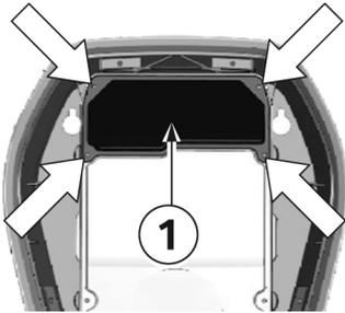
1. Undo the four screws used to secure the termination panel cover **1**.
