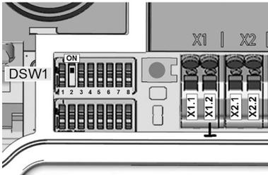
The use of the domestic connection monitoring function with RS485 meters must be selected using a DIP switch setting and does not come into effect until the Wallbox has been restarted. If no meter **5** is found when the ModBus function has been enabled, the charging current is reduced to 10 A.
